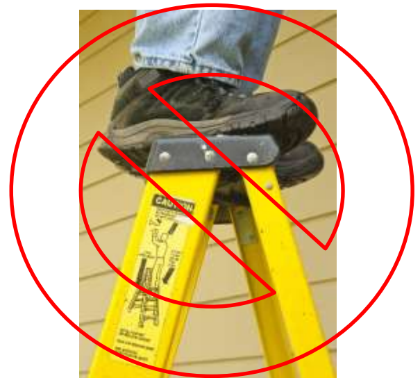
Figure 1 IMPROPER ladder usage
